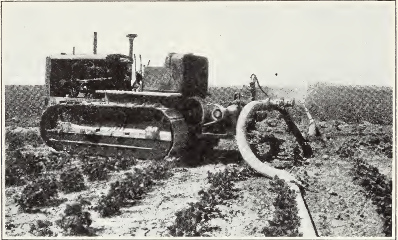
Fig. 20.—Large portable pumping plant: 50-hp. Diesel tractor operating 5-inch centrifugal pump; two lines of pipe totaling 2,480 feet with 6-foot sprinklers. The total discharge is approximately 1,100 gallons per minute.
